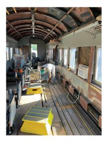
Work continues on 1158. Our progress slowed down a little bit over the summer when some resources had to be diverted over to work on 1341's roof edge. The steel floor in 1158 is now finished and awaiting concrete. Issac and John spent many hours welding the sheet metal together, as well as welding in the C channel supports that give the floor additional support.
