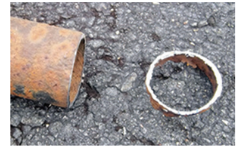
(Left) Sharp, rusty, bent, and flattened end of "W" sign was cut off to get to good metal (Right) Sharp, rusty, and corroded end of "RR" sign was cut off to get to good metal
