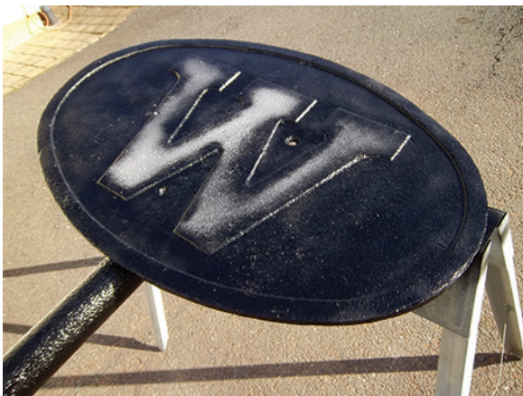
Rust inhibitor, primer, and black paint applied
