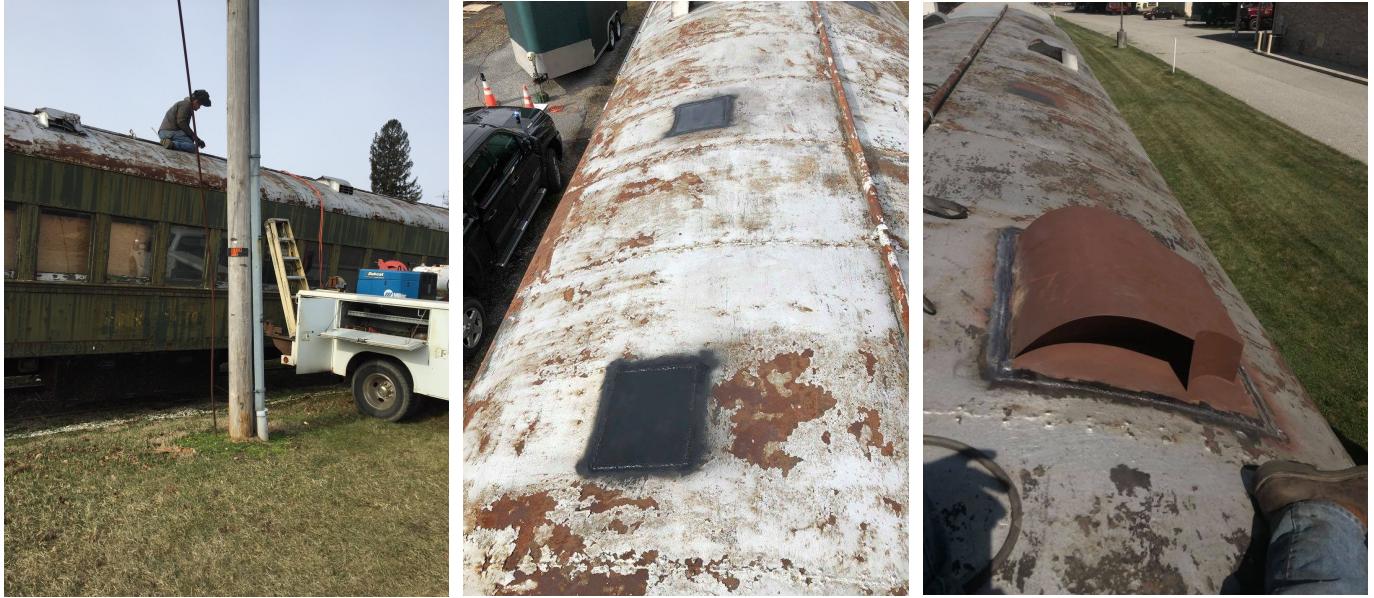
Left: Contract Welder on the roof, Middle: Completed Patch Repairs, Right: Reproduction Roof Vent Installed
