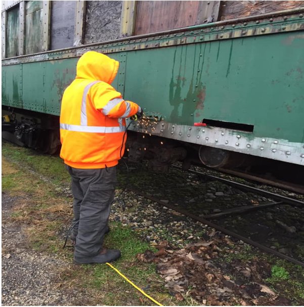
Left: Volunteer cutting out bad spots in the side sheets, Right: Volunteer grinding down welds Bottom: Volunteers Welding in Patches & Blending freshly
