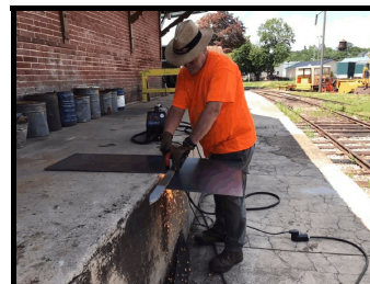
Left: Jim Kuhlman cutting a sheet of steel using the Friends plasma cutter.
