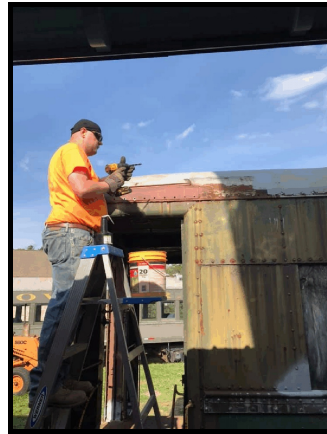
Left: David Collison installing buttonhead screws on the roof of coach #1158.
