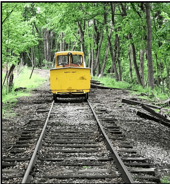
A work train approaching the iron bridge from the east. The motorcar is in the back pushing the railroad's tool car to the work-site. Photo by David Williamson.
