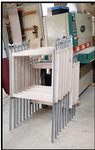
New coach window frames being fabricated. Photo by Custom Woodworks.
