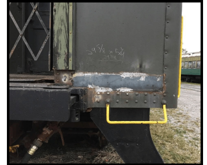
Above left: A section of coach #1341 being prepped for welding of a patch. Above right: The replacement patch welded in place.
