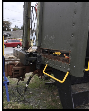
Above left: A section of coach #1341 being prepped for welding of a patch. Above right: The replacement patch welded in place.
